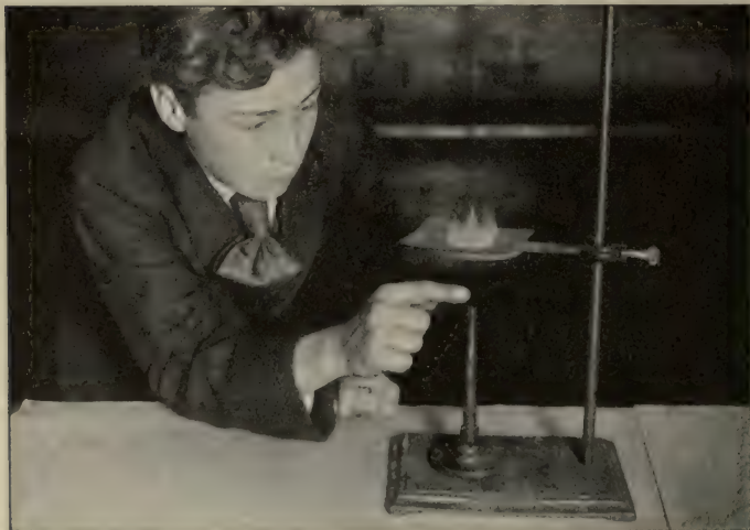
FIG. 171. Why doesn't the flame above the wire gauze set fire to the gas below?
